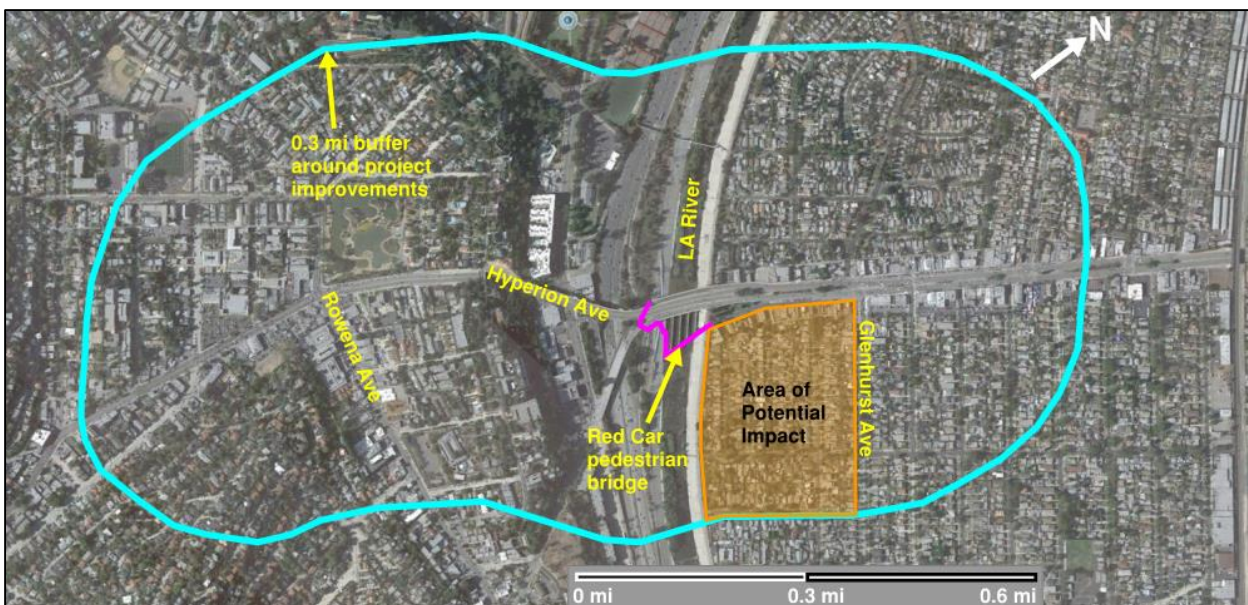
Figure 5 Area Potentially Impacted by Lack of Sidewalk on East Side of the Hyperion Bridge
