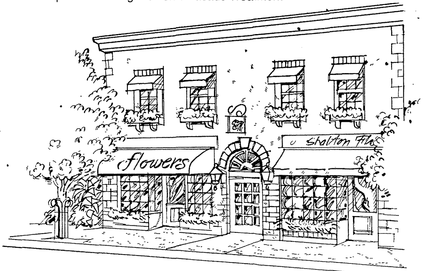
Figure 2. Transparent Building Element / Facade Treatment
