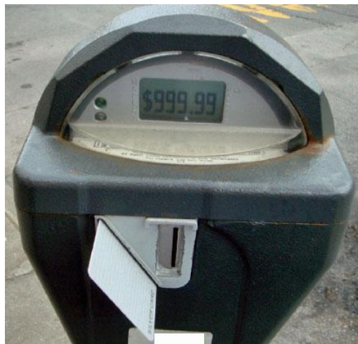
Figure 1: “Hacked” parking meter showing $999.99 balance on smart card
