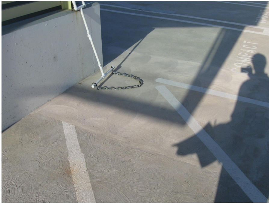
Photo 58 – Delaminated area found by chain drag
