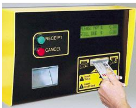
Figure 3 – Exit Reader of a Card In/Card Out System
