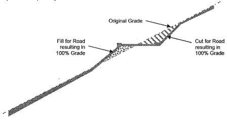
In addition, staff conducted an analysis of all the single-family zoned lots in the Hillside Area and found that only 0.14% of the area is greater than 45% slope. Consequently, after discussions with LADBS, staff recommends removing the prohibition of grading on extreme slopes (greater than 100%).
