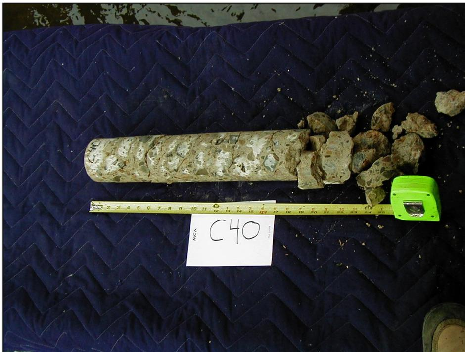
**Figure 1-7 Concrete Core Sample Showing Damage Caused by ASR**
