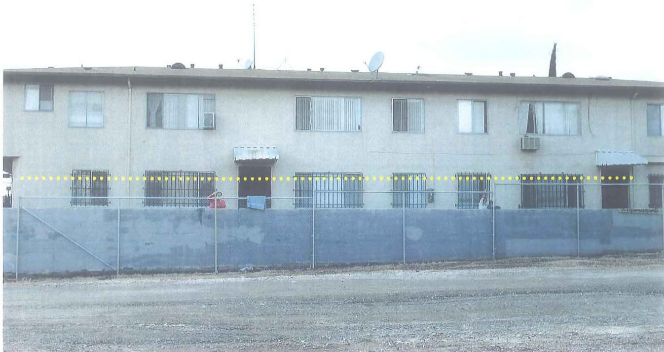
Dotted line delineates 10-feet above grade. First floor units at 5248 Virginia Ave. would have minimal noise mitigation with a 10-foot attenuation blanket. Second-floor units would have no mitigation. Note below photo of 10-foot height of measuring tape, replicating height of sound blanket.
