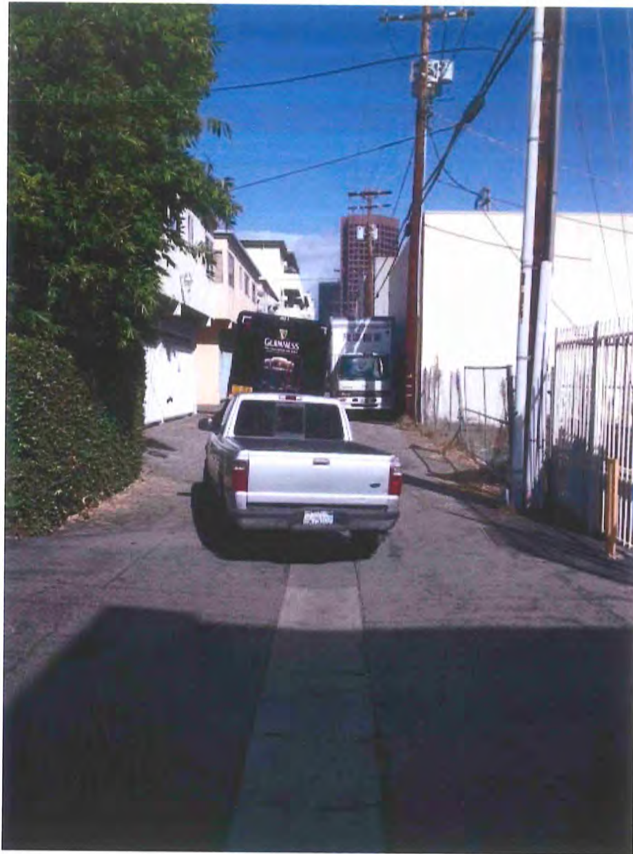
A variety of vehicles use the alley. Note the variations in the width of the alley. The pick-up truck is delayed while the eastbound truck is trying to squeeze by the parked truck. The utility pole on the right hand side is at the western boundary of the proposed project where the alley width is 15 feet.
