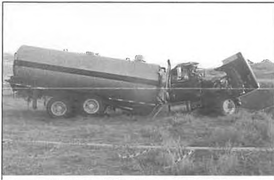
The point here is that if the truck hadn't run into the ravine - if the truck had lost its momentum rolling through the field or otherwise been brought to a controlled stop - the operator may have survived this accident unharmed.
