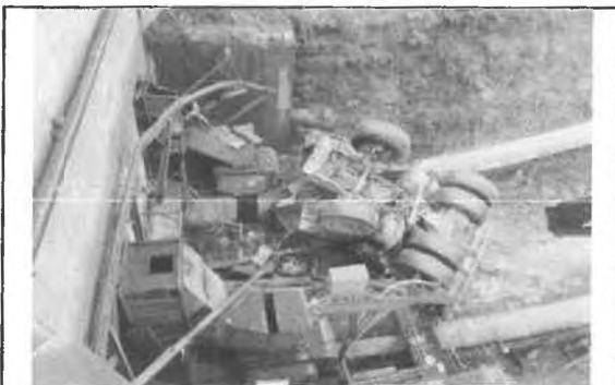
The accident investigation also revealed that there was no braking effort available from the front service brakes because of a leaking seal. The rear service brakes were found to be capable of providing 78 % of their design braking capacity.
