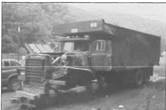
The 20-ton capacity truck was found to have been loaded to about 45 tons. In addition, the driver apparently was not adequately trained on the operation of the truck and the escape-ramp safety features.
