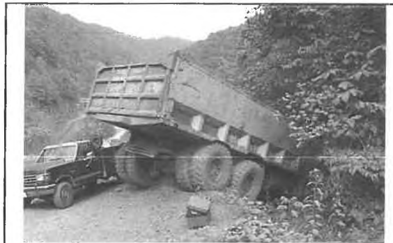
The accident investigation revealed that the front brakes were inoperative and there was no braking force from the right rear brake.
