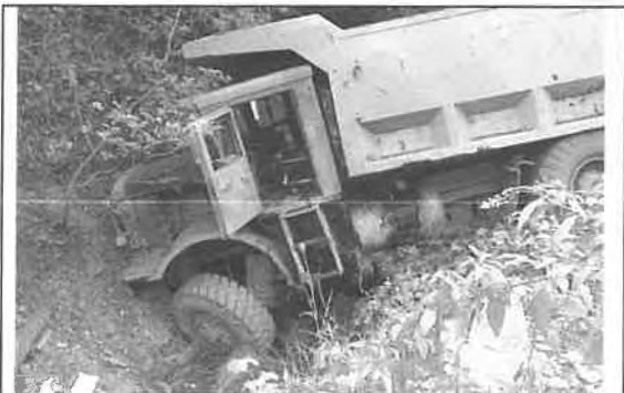
The conclusion on this accident was that the deficient and uneven braking, combined with speed too fast for the wet and steep-road conditions, resulted in the truck leaving the haul road. The victim was not wearing a seatbelt and was thrown through the windshield.
