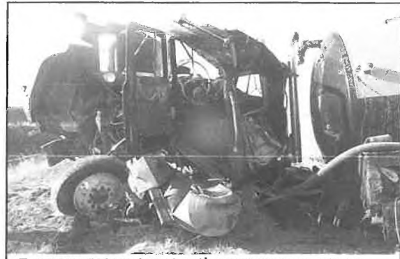
The accident investigation revealed that the truck's front brakes had been removed and the rear brakes were defective. Rear brake problems included a severe air leak, oversized brake drums, and excessive pushrod stroke.
