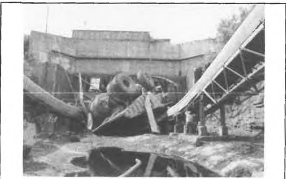
The truck went over the wall and ended up here. The victim was not wearing a seatbelt. The accident investigation revealed that the electrical retarder had failed to operate because of a problem with the contacts between the brushes and the commutator.
