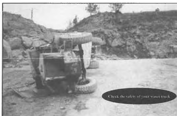
Several fatal accidents have occurred in recent years involving water trucks. This one occurred as the water truck rounded a curve while descending a 7 to 9 % grade. The victim's regular job was in quality control and he only occasionally drove the water truck.
