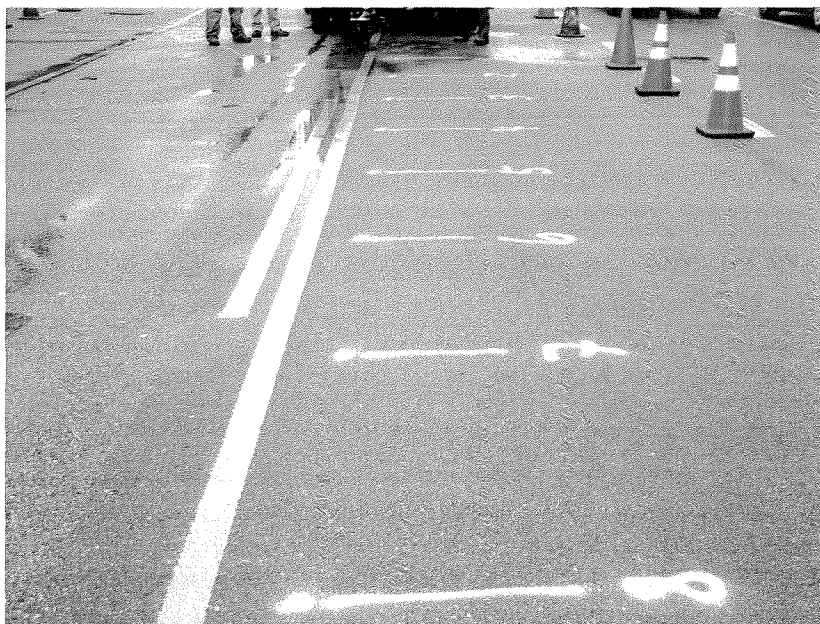
Figure 3: Shows FWD to be measured in a control area with consistent Asphalt thickness structure.
