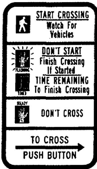
**Pushbutton Detector Unit Signs**
