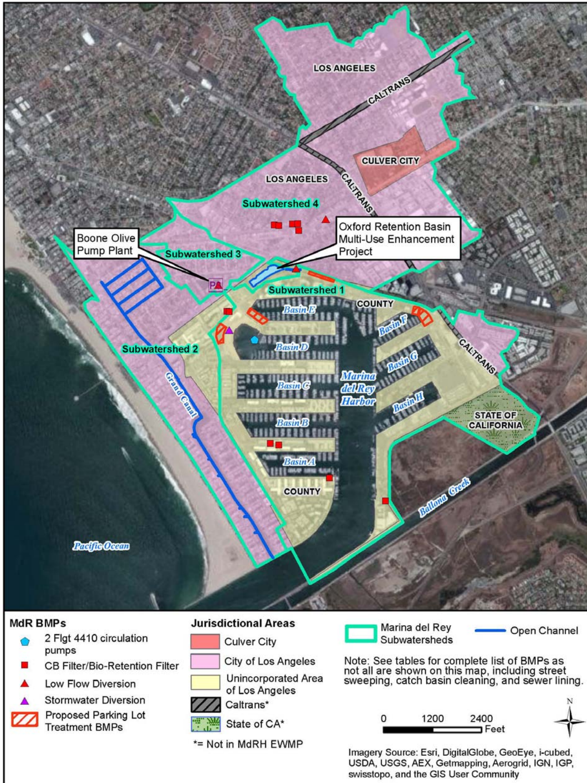
Figure 4-1: Existing Structural MCMs within MdR Watershed
