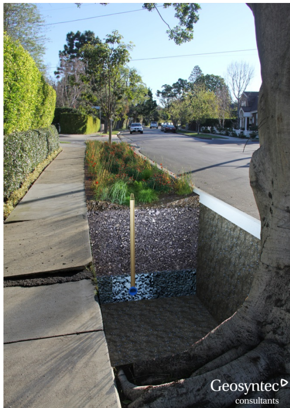
Figure 4-23 Section View of Bioretention with Underdrain
