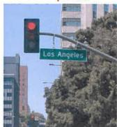
A rest in red signal timing operation keeps the signal in the red phase until drivers slow and activate the green signal phase at the intersection, helping to reduce vehicle speeds during off-peak periods.
