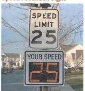
Speed feedback signs electronically display a driver's speed to encourage obeying speed limits.
