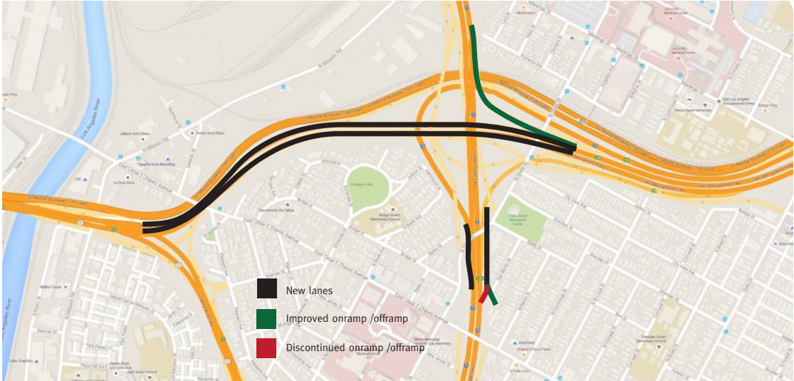
Figure 11: North Interchange Design: I-5 and I-10
