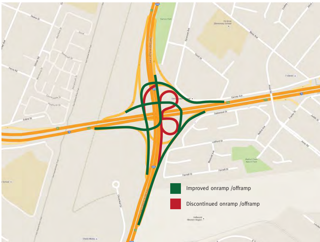
Figure 16: Interchange Design: I-10 and I-605
