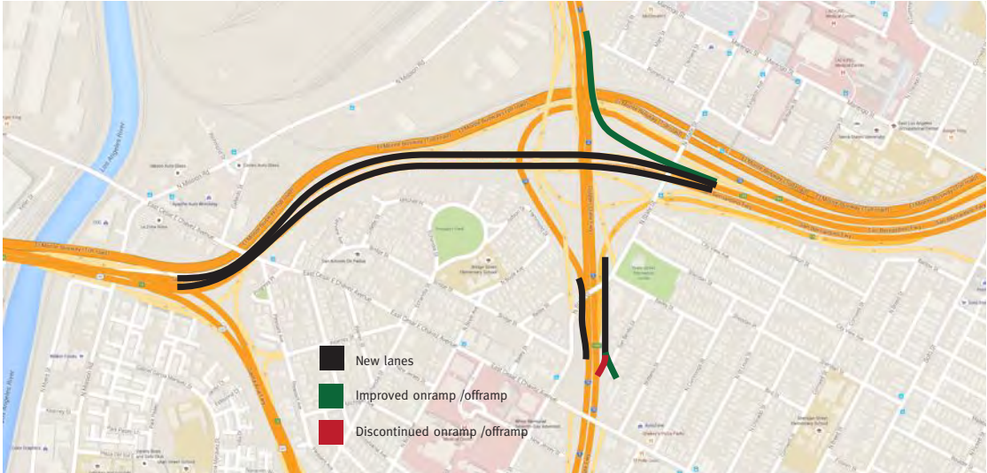
Figure 11: North Interchange Design: I-5 and I-10
