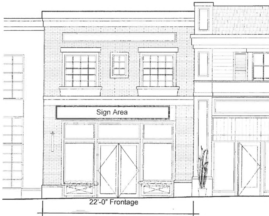
Figure 7 — Typical Tenant Storefront Wall Sign
