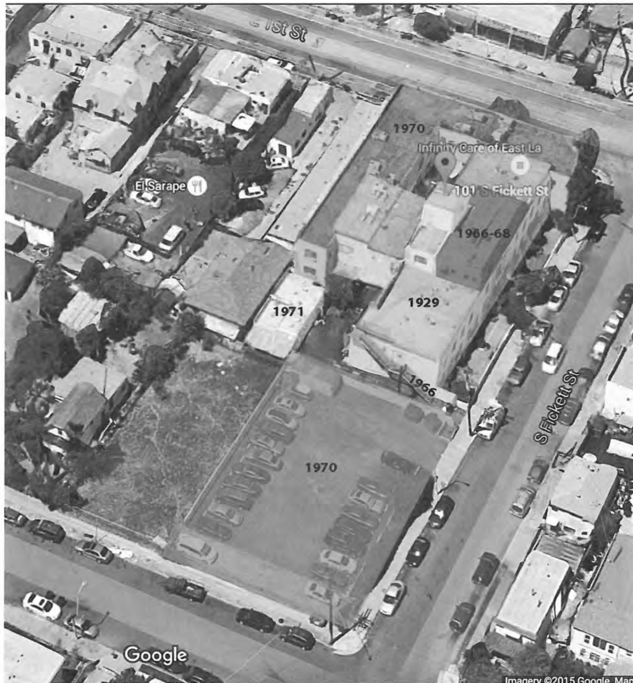
Fig. 4: Schematic Diagram of Japanese Hospital, indicating dates of construction or alteration to the various components of the building. (Little Tokyo Historical Society, 2015)
