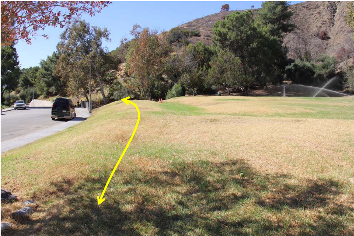
Site 1: Looking west across the front of the park. The double yellow arrow points out where 160 linear feet of K-rail has been recommended to be placed in order to prevent debris flow from entering the street.
