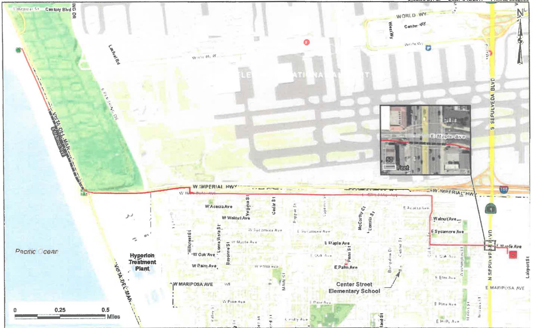
Figure 2-2 Terrestrial Conduit Route Los Angeles Trans-Pacific Telecommunications Cable Hub
