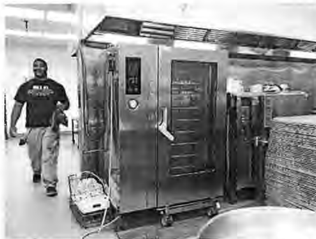
An OUSD Nutrition Services worker walks by an Angelo Po combination oven at Prescott's central kitchen. These ovens will allow schools to prepare fresh, scratch-made food for cafeteria meals. Photo: Sarah Han
