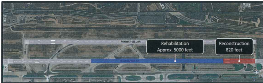
Figure 5 – Runway 6R-24L Rehabilitation
